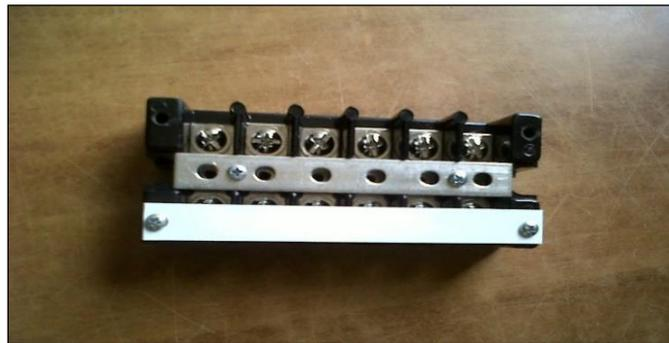
**Figura 4. Bornera cortocircuitable**
